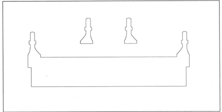
These components can be used with scratchbuilt models, our own components or as replacements for the plastic components supplied with the Ian Kirk kits. Note: the thickness of the Kirk solebars means that they will need to be thinned to clear the etched truss posts, and the etched truss posts reduced in width.
