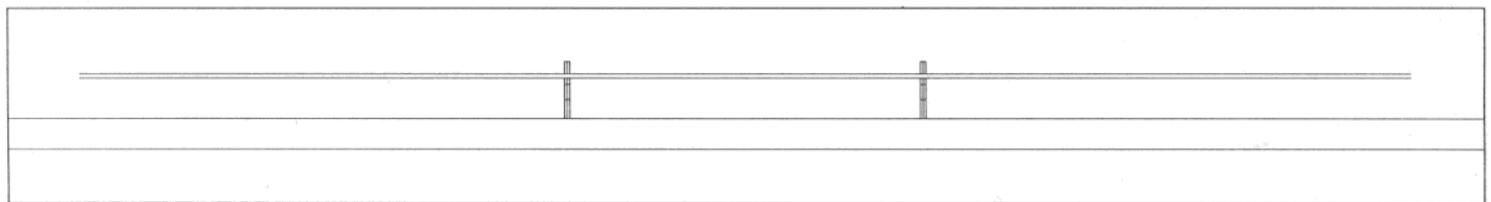
Glue or solder the truss bars onto the truss posts followed by the etched 'nuts' (Part B) trapping the truss bars. When fixed, take the pliers and twist the etched bars next to the truss posts through 90 degrees, so that the turnbuckles are now vertical. (Although not shown on the drawing repeating the process for the central portion of the truss bar improves their appearance).
