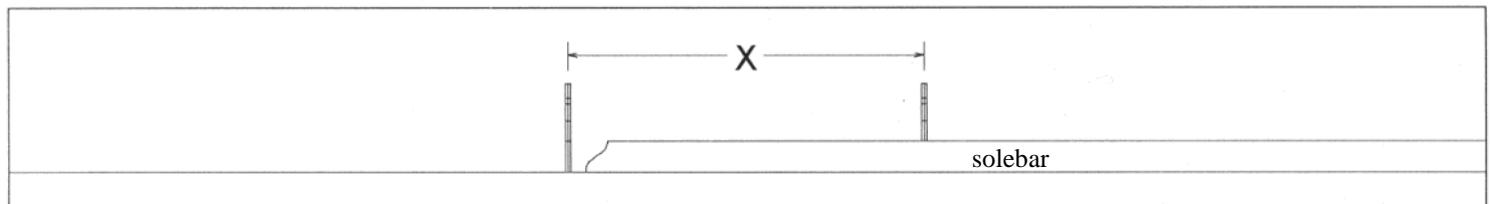
Glue or solder the truss posts in place on the underside of the floor, 40mm between centres for 60'0" underframes and 34.3mm for 51'0" underframes. Tip: Mark the positions on the floor then check the measurements against the truss rodding fret before final fixing. Remove the truss bars from the fret and clean off any tabs by holding the fret in a fine pair of pliers next to the tab to avoid damaging it.
