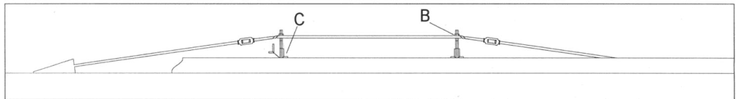
Bend the bars down so that they meet the floor of the vehicle behind the solebars. Take the etched needle beams (Part C) and using a blunt compass point emboss the rivets using the half etched holes as a guide. Only the outer sets of rivets are required when two truss posts are being used. Bend the beams through 90 degrees with the half etched fold line on the inside of the fold and fix to the truss posts, across the solebars, as shown.
