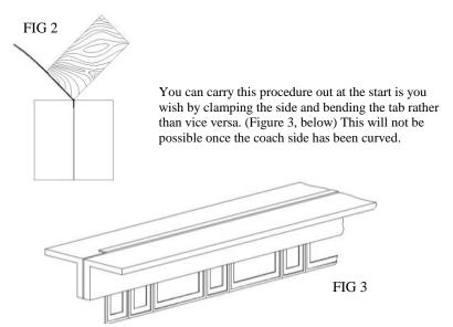
You may need to remove about 2mm of the flange at each end if you are using a proprietary coach as a base, such as the Hornby Gresleys. This is to allow the side to fit between the ends - it also helps to centre the side on the end/roof frame.
